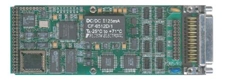
The M395 features 16 analog voltage outputs, integrated on the ANSI certified M-module standard. The digital-to-analog converters have a resolution of 12 or 16-bit.
